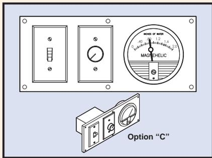
Magnehelic Gage is surface mounted on a flat control panel with On/Off switch and variable speed control.
