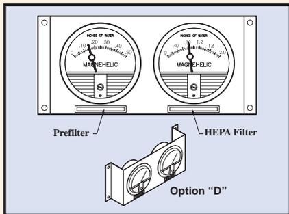
Dual Magnehelic Gages measure prefilter and HEPA/ULPA filter resistance.
